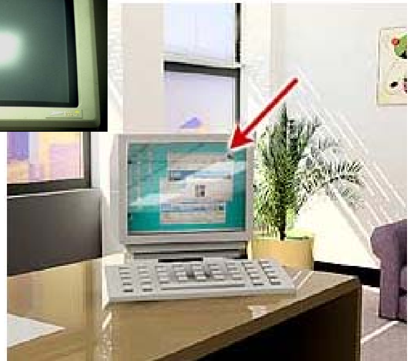
Reflected glare on the computer screen from ceiling luminaires
